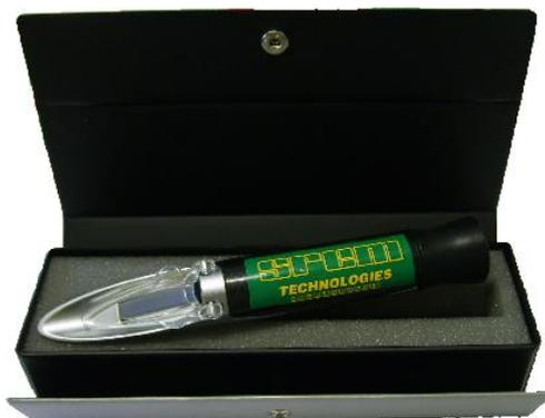
The hand-held refractometer is a simple device to control the concentration of emulsifier.
